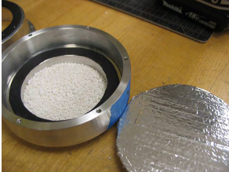
Photo No. 3 Test Cup Desiccant Chamber Detail
